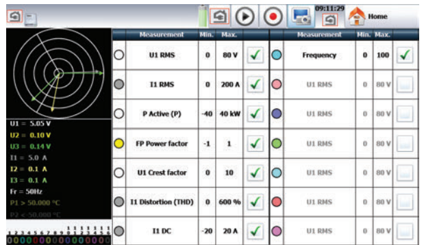
Select which measurements are displayed on screen
