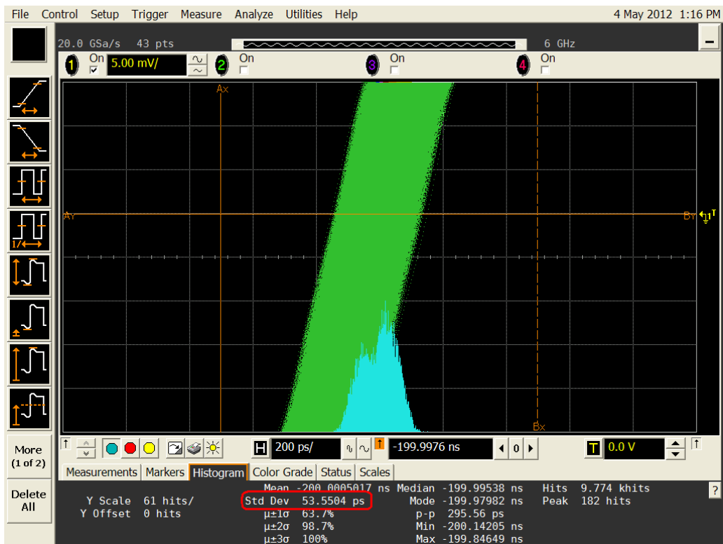
Figure 4. Jitter measurement on DDS signal.
