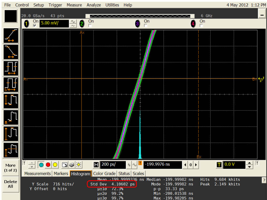
Figure 3. Jitter measurement on Trueform signal.
