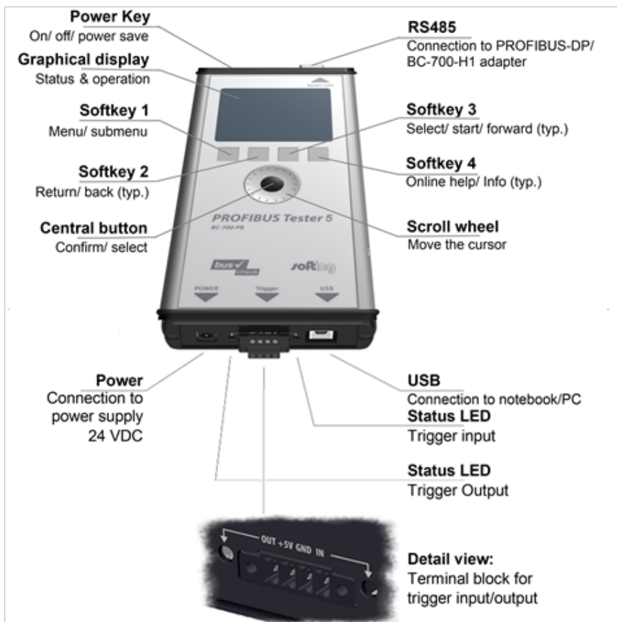
Figure 10: Connectors, buttons and status displays on the BC-700-PB
