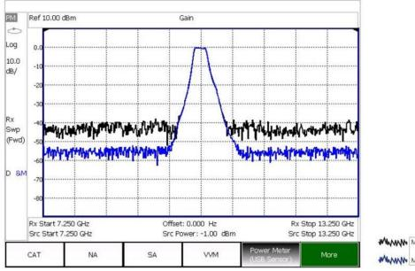
Masured using U2021XA power sensor Man Measured using U2002A power sensor
