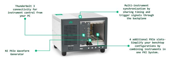
With the PXI waveform generators, generate standard functions and user-defined, arbitrary waveforms as part of a PXI system. The PXI Waveform Generator bundles feature up to 2 output channels with up to 80 MHz bandwidth,  $\pm$  12 V output range and 800 MS/s maximum update rate.
