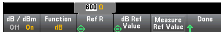
Figure 6. Automatic scaling provides a convenient logarithmic readout relative to a user-set reference
