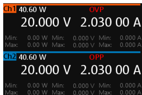
Figure 5-14: Indicator of OVP/OPP when tripped
