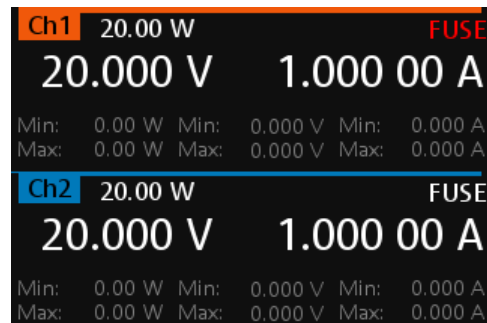
Figure 5-11: Fuse indicator on respective channel
