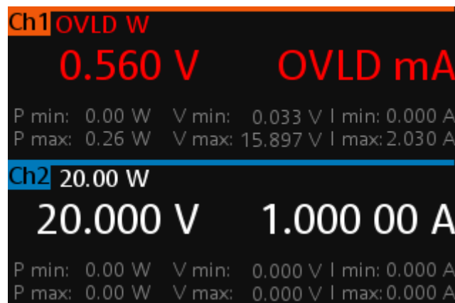
Figure 5-6: Display of OVLD indicator when current > 205 mA at Ch 1
