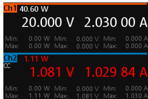
Figure 5-3: Output of Ch2 in CC mode
