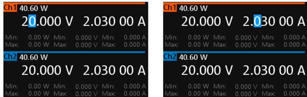
Figure 5-2: Voltage and current settings in the instrument
