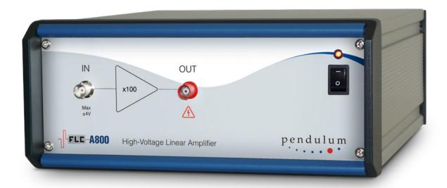
The Pendulum Instruments High Voltage Linear Amplifier A800 has a fixed amplification of 100 times and capable of bipolar high voltage output of ±400V. Any signal source with amplitude up to ±4 V can be used as an input device. The input amplitude should normally be kept within ±4 V. The A800 High Voltage Linear Amplifier is equipped with a microfuse rated at 40 mA, which will be blown if the input voltage exceeds 500% of the maximum.
