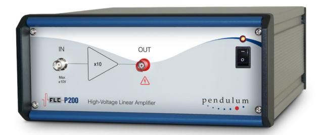
The Pendulum Instruments High Voltage High Current Linear Amplifier P200 has a fixed amplification of 10 times and capable of bipolar high voltage output of ±100V. Any signal source with amplitude up to ±10 V can be used as an input device. The input amplitude should normally be kept within ±10 V. The High Voltage High Current Linear Amplifier P200 is equipped with a microfuse rated at 40 mA, which will be blown if the input voltage exceeds 300% of the maximum.
