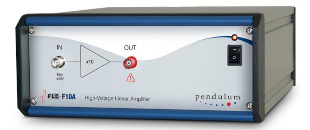
The Pendulum Instruments High Voltage Linear Amplifier F10A has a fixed amplification of 10 times and capable of bipolar high voltage output of  $\pm 100$ V. Any signal source with amplitude up to  $\pm 10$  V can be used as an input device. The input amplitude should normally be kept within  $\pm 10$  V.
