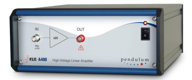
The Pendulum Instruments High Voltage Linear Amplifier A400 has a fixed amplification of 20 times and capable of bipolar high voltage output of ±200. Any other signal source with amplitude up to ±10 V can be used as an input device. The A400 High Voltage Linear Amplifier is equipped with a microfuse rated at 40 mA, which will be blown if the input voltage exceeds 300% of the maximum.
