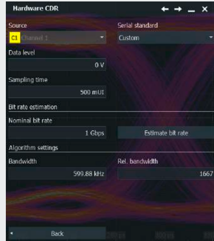
The configurable CDR of the R&S®RTO6 supports data rates up to 6 Gbit/s for data eye analysis.
