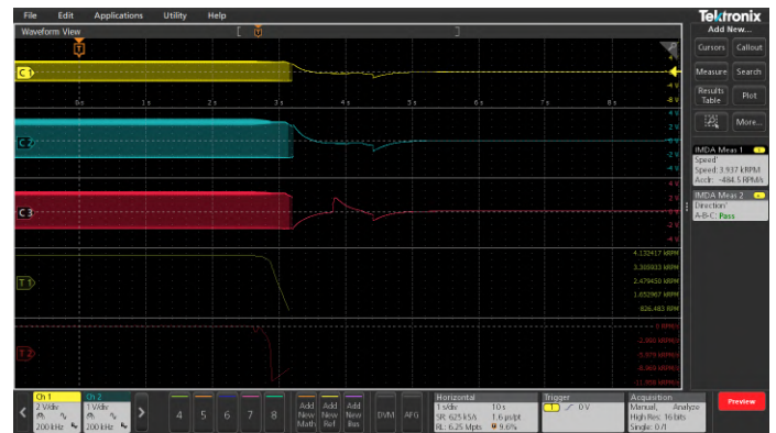
Time trend plot displaying deceleration of a motor into a stop state.
