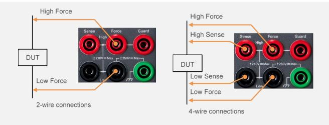
Low current measurements (< 1 nA) require guarding to prevent leakage through the measurement cable. The schematic shown below provides a simplified overview of the guarding technique. Guarded measurements require the use of triaxial cables. A follower (x1) buffer amplifier keeps the guard conductor at the same potential as the center conductor. Since there is no voltage difference, no current can flow from the center conductor to the guard.
