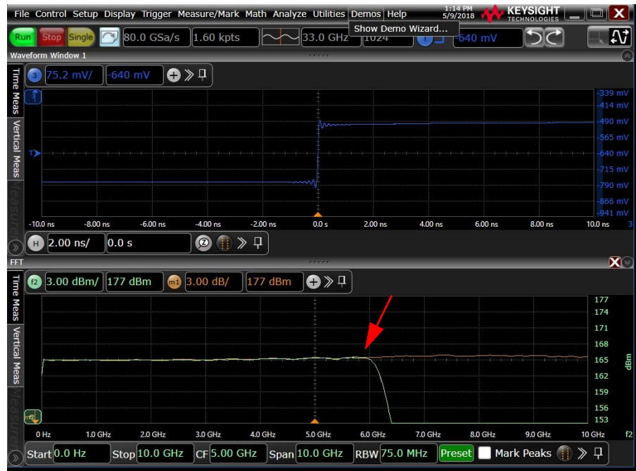
Figure 34 Frequency response of the N7024A probe with the N7022A main cable
