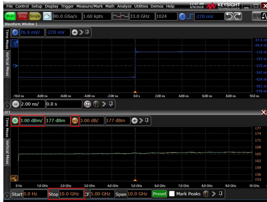
Figure 30 Frequency response of the Cal Out step through the attached coax cable
