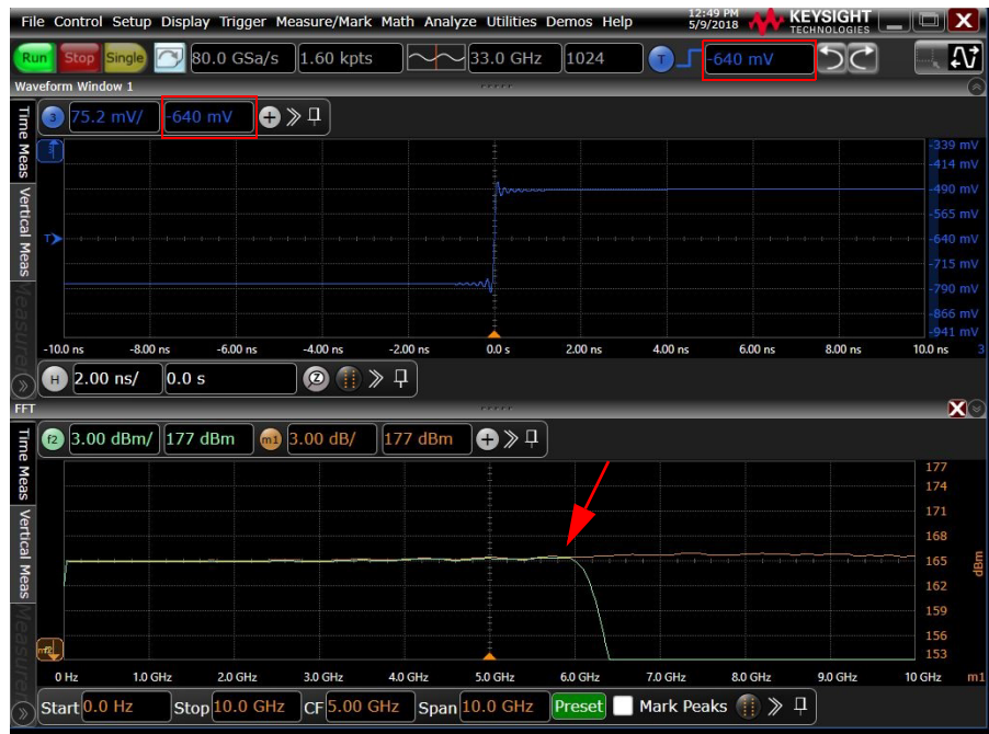
Figure 32 Frequency response of the N7024A probe
