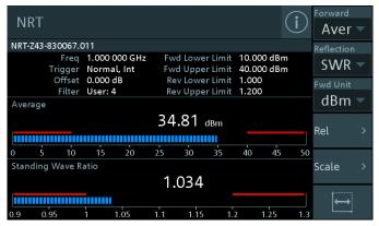
Analog bar graph with configurable limits
