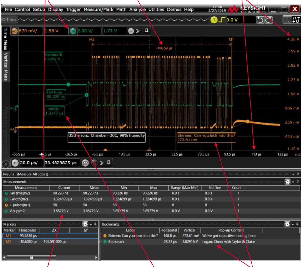
Select from over 50 automatic drag and drop measurements.
