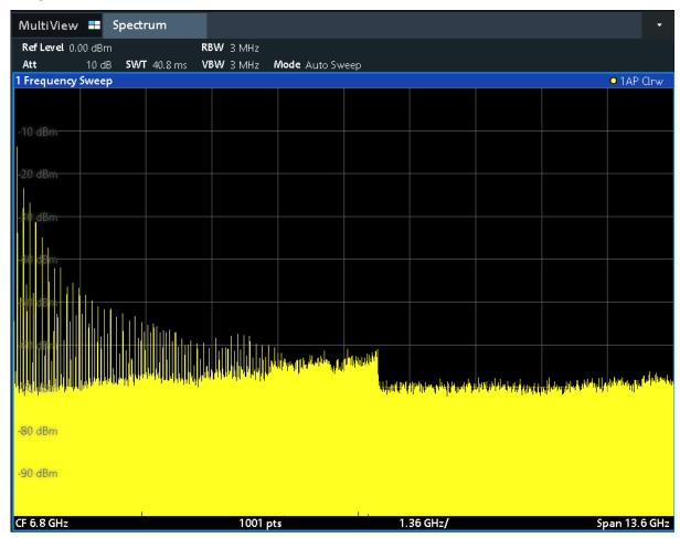
Figure 7-1: Calibration signal as RF input
