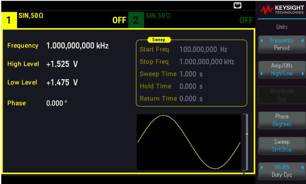
2. Press [Parameter] > **High Level**. Using the numeric keypad or knob and arrows, select a value of 1.0 V. (If you are using the keypad, you will need to select the V unit softkey to enter the value.)
