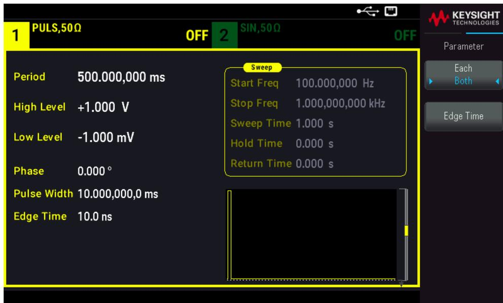
Press **Edge Time** to set the edge time for both the leading and trailing edges to 50 ns. The edge time represents the time from the 10% threshold to the 90% threshold of each edge.
