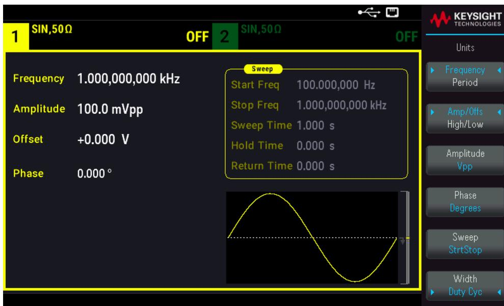
2. Press [Sweep] > **Start Freq** or **Stop Freq**. Use the numeric keypad or the knob and arrows to set a desired value. If you use the keypad, select a prefix unit to finish.
