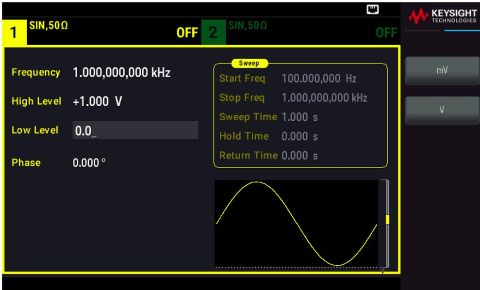
These settings (high-level = 1.0 V and low-level = 0.0 V) are equivalent to setting an amplitude of 1.0 Vpp and an offset of 500 mV.
