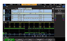
Figure 19. Multi-bus time aligned decode.
