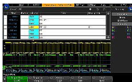
Figure 15. I2C decode and trigger.
