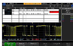
Figure 17. CAN-FD decode and trigger.
