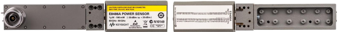
Figure 1. E8486A-100 comes without built-in EEPROM with dynamic range of -30 to +20 dBm. Users need to pre-enter calibration factors printed on the back of the sensor into the power meter.
