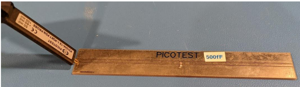
Fig. 15 - TDR Measurement Setup for 500fF Capacitor with the P2104A Probe.
