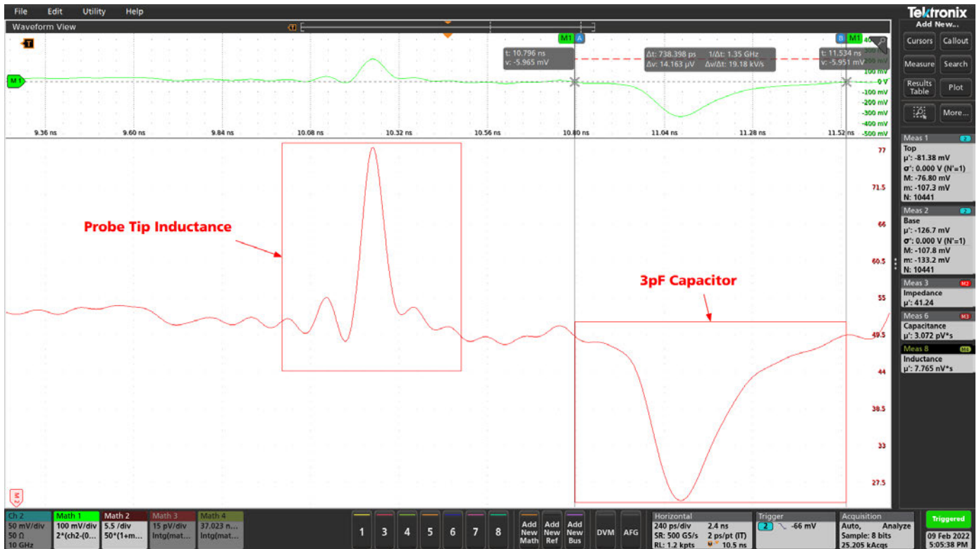
Fig. 14 - TDR Measurement Result of the 3pF Capacitor with the P2104A Probe and J2154A TDR.
