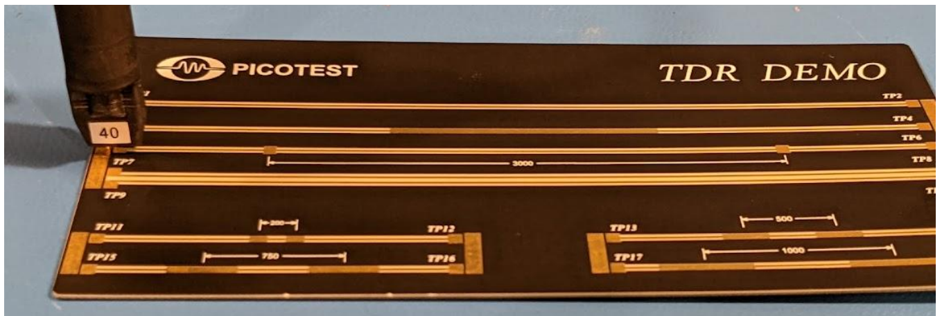
Fig. 22 - TDR Measurement Setup with Picotest Demo Board TP5 Trace with the P2105A Probe.
