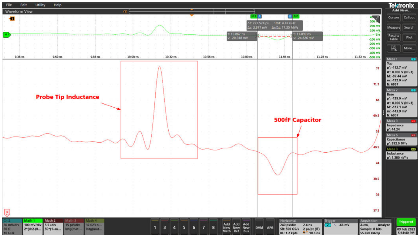
Fig. 16 - TDR Measurement Result of a 500fF Capacitor with the P2104A Probe and J2154A TDR.
