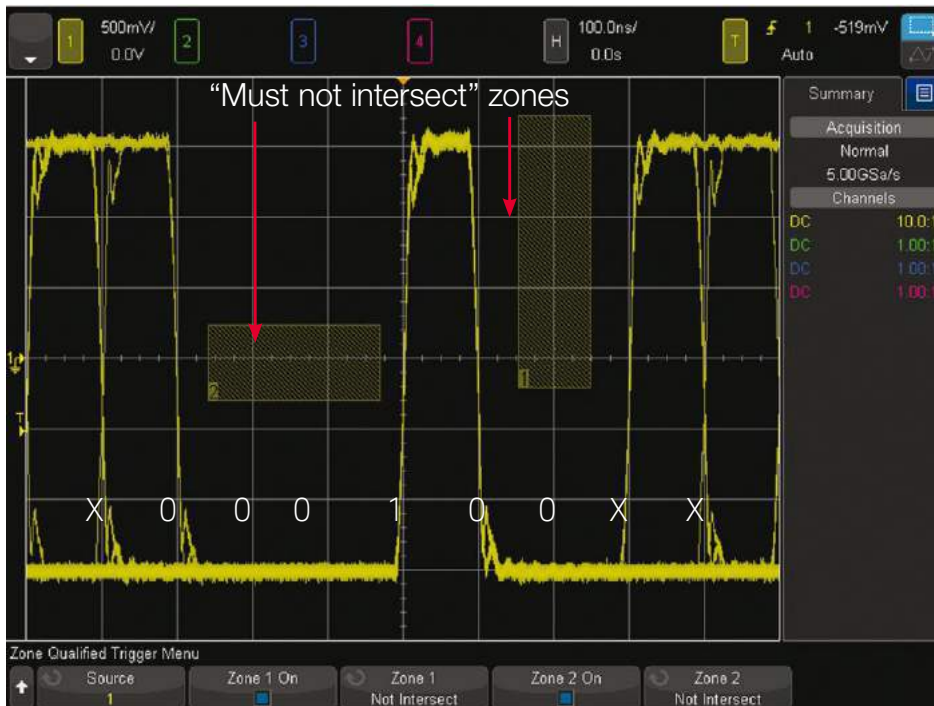
Figure 8. Triggering on isolated “ones” using two “must not intersect” zones along with a rising edge trigger.
