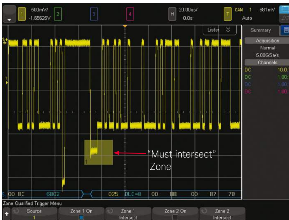
Figure 11. Using Zone Trigger to synchronize on just frames that include arbitration.
