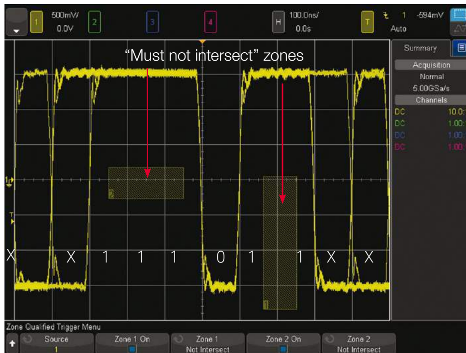
Figure 9. Triggering on isolated “zeros” using two “must not intersect” zones along with a falling edge trigger.
