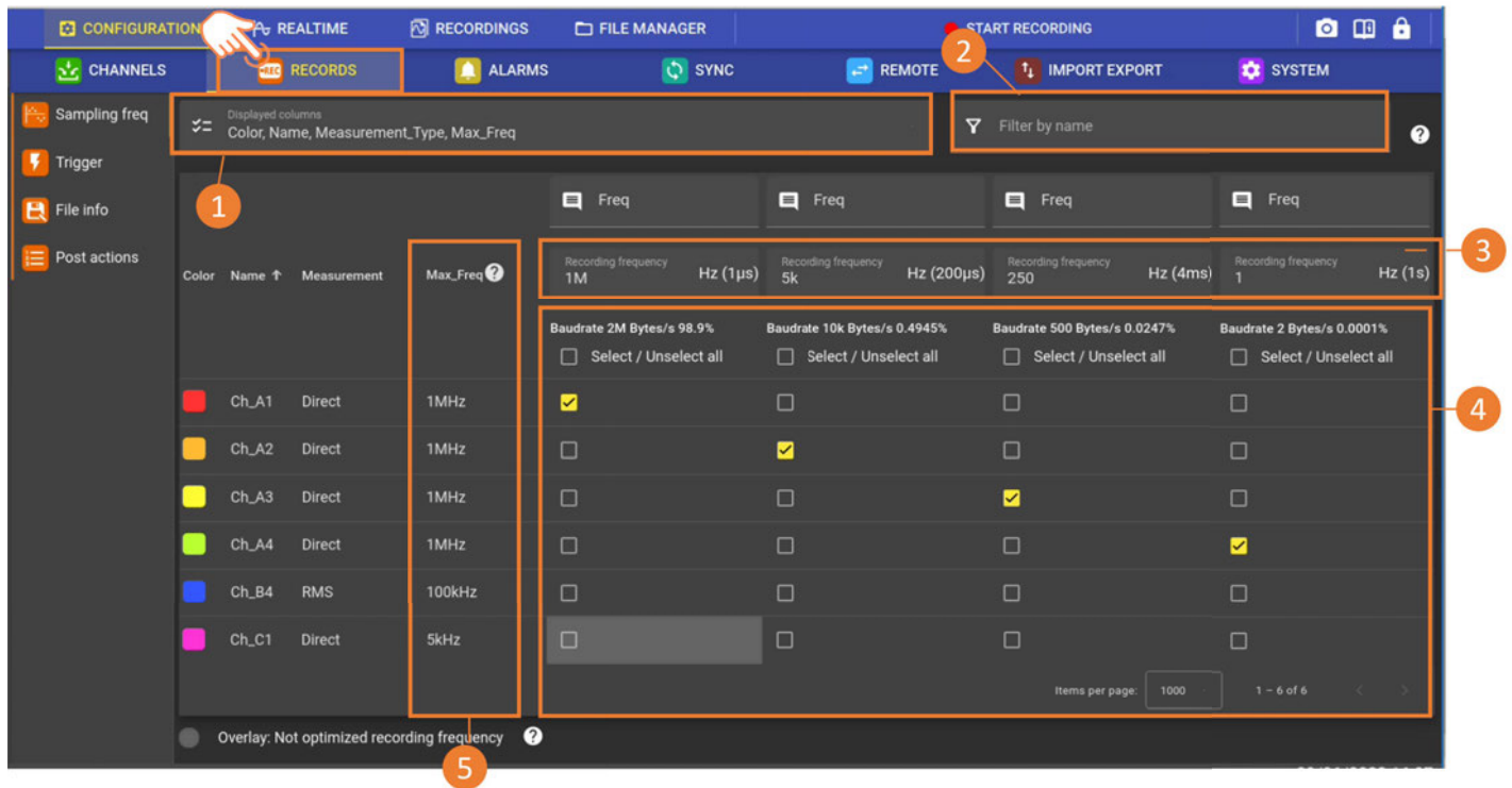
FIGURE 3.11 : Setting recording frequencies
