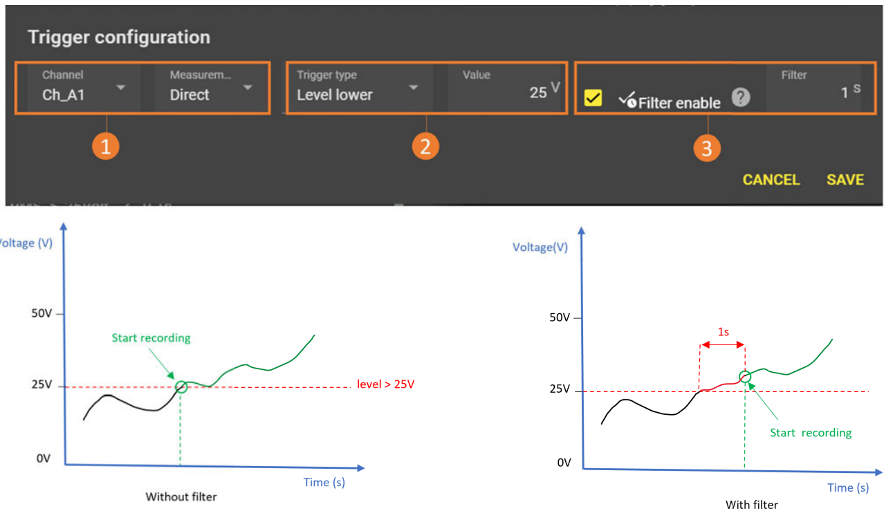
FIGURE 3.14 : Trigger on level
