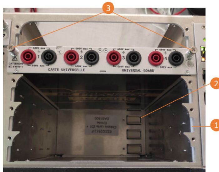
FIGURE 3.1 : Add an acquisition module
