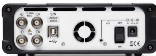
Figure 3 - Rear panel of the AS108
