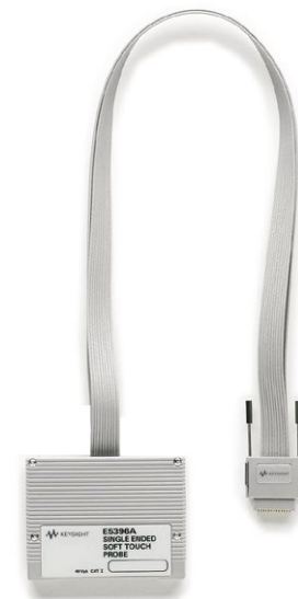
E5396A 16-channel soft touch connectorless probe
