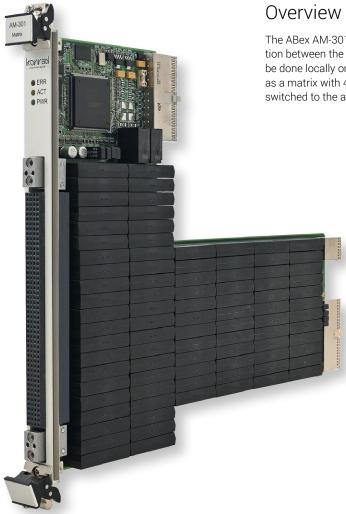
The ABex AM-301 is a 172x4 matrix designed as a universal connection between the test points and the measuring instrument. This can be done locally or via the ABex. The ABex AM-301 can be configured as a matrix with 4 or 8 busses. The internal matrix busses can be switched to the analog bus.
