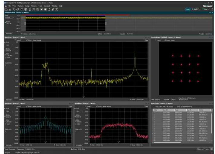
Analyze both wide and narrow bandwidths simultaneously. On the same oscilloscope channel of the 6 Series MSO, a 64QAM signal and a pulsed radar signal are captured using Source 1. For detailed analysis, Source 2 zooms in on the radar signal, while Source 3 focuses on the 64QAM signal.
