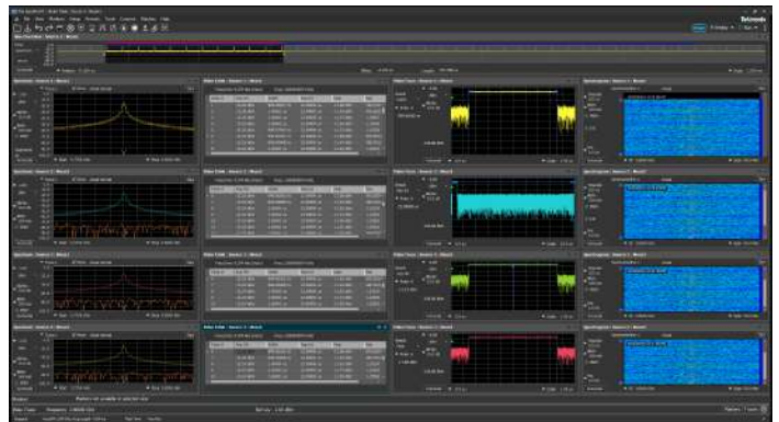
Four pulse trains are captured and analyzed simultaneously with time-correlated markers, pulse table, and pulse trace displays used to gain insight into the signal behavior across channels over time.
