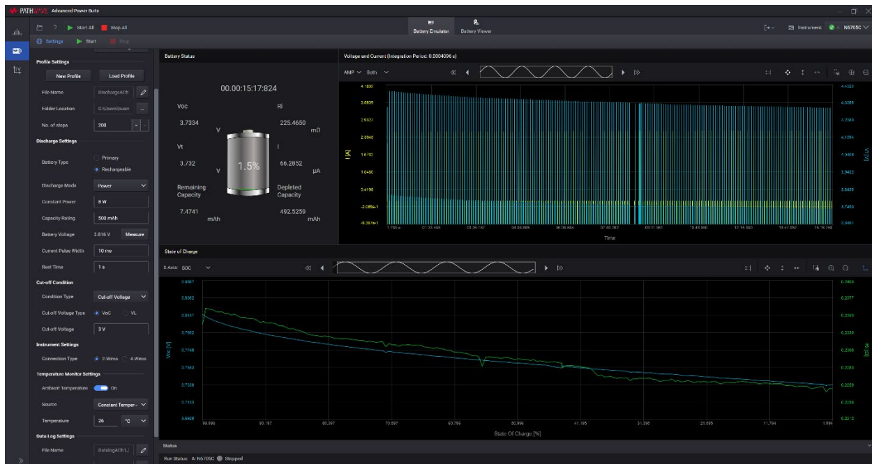
Figure 9. PW9254A creating a battery profiler with ambient temperature, constant power discharge features
