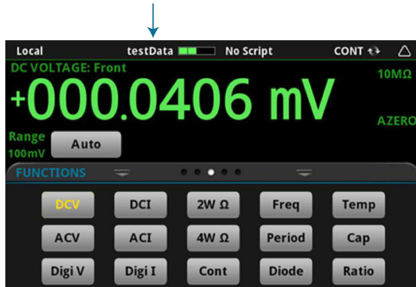
Figure 119: Active buffer indicator
