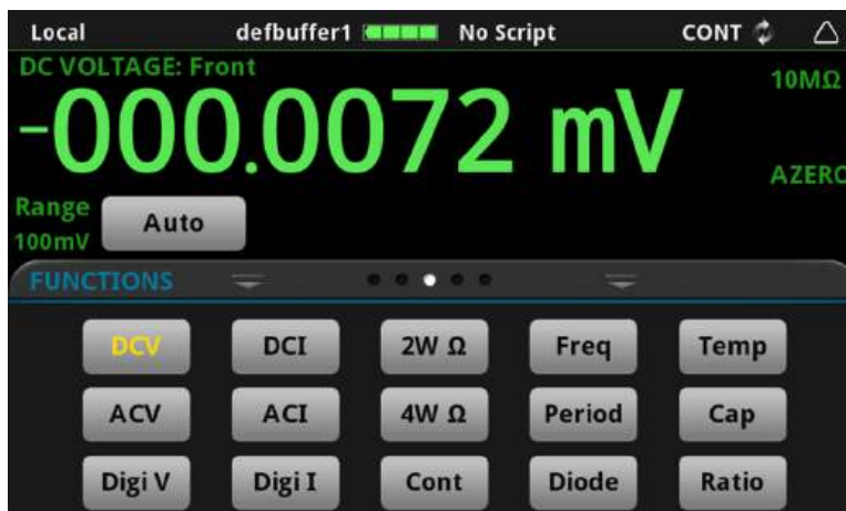
Figure 28: DAQ6510 home screen - front
