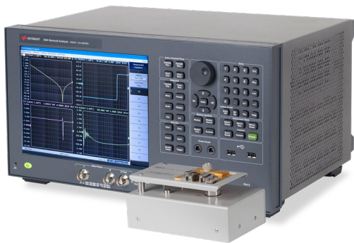
Port-1 reflection method using 16201A terminal adapter and 16092A 7 mm type fixture
