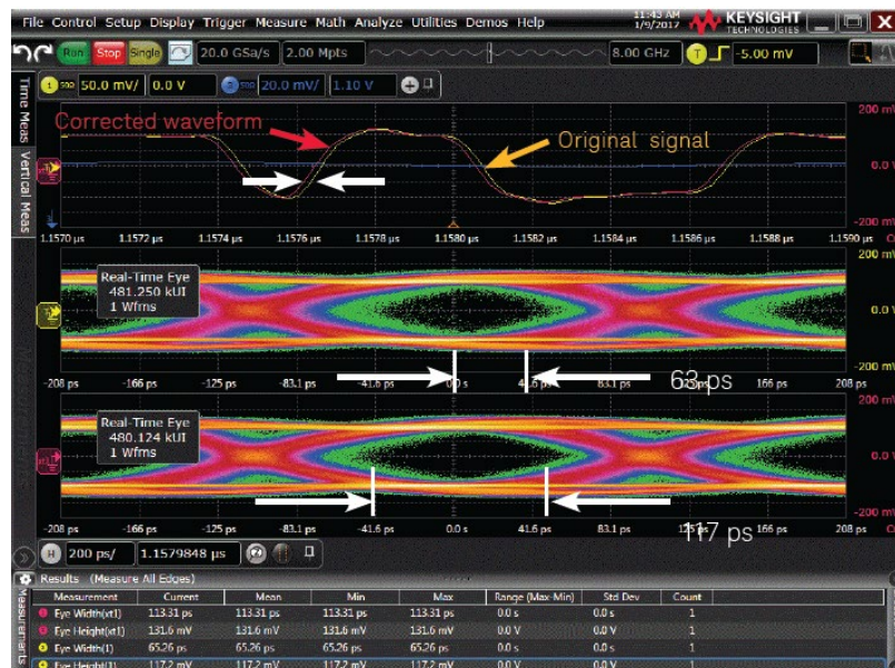
Figure 21. Expanded timebase view of the FPGA serial data with and without the effects of the DC supply noise.
