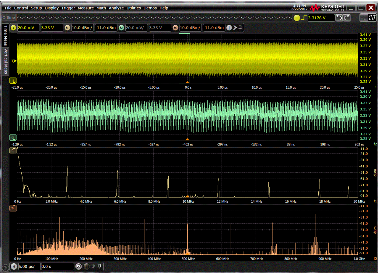
Figure 22. N7020A Power Rail Probe and S-Series High-definition oscilloscope measuring the noise on a 3.3 V supply.
