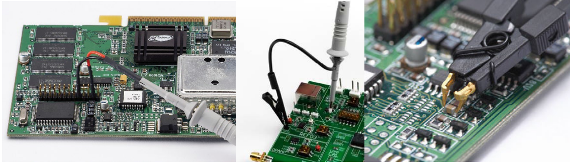
Figure 12. (left) Dual lead adapter: The dual lead adapter allows you to easily connect the N7023A power rail probe browser to popular 0.1" pin headers with 0.025" square pins. This dual lead adapter has no shorting hazards since all external metal surfaces are insulated. (middle) 15 cm ground lead: This ground lead can be used to reach grounding locations that are farther away from the probing location than can be reached by the ground spring. (right) Dual lead adapter with Micro SMD clip: The Micro SMD clips were designed to provide fast and convenient hands-free probing of surface mount capacitors. The Micro SMD clip is used in conjunction with the dual lead adapter.
