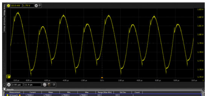
Figure 1. Using the N7020A power rail probe, with 2 GHz bandwidth and 50 k \Omega DC resistive loading, to see the AC and DC components of a DC power rail.
