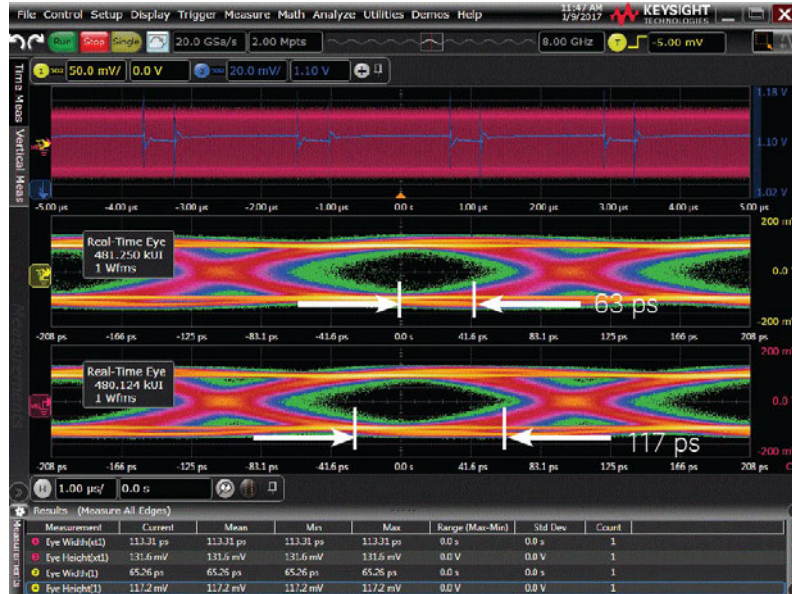
Figure 20. Results from the D9110POWA PI analysis application showing the eye diagram of the FPGA serial data before and after the effects of the DC supply noise are removed.
