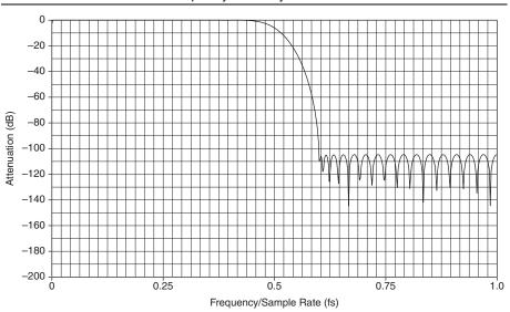
Figure 2. NI 4461/4462 Digital Filter Input Frequency Response with Low-Frequency Alias Rejection Disabled
