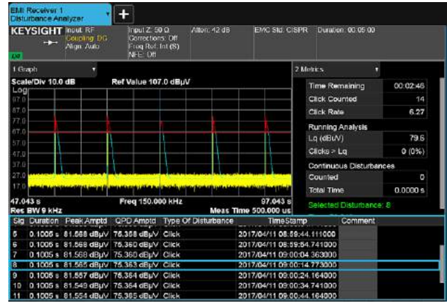
Figure 8. Simplify and automate data collection, analysis, and report generation for click measurements
