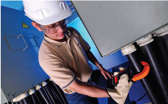
Figure 2. Large jaw clamp opening of 52mm / 2 inches
