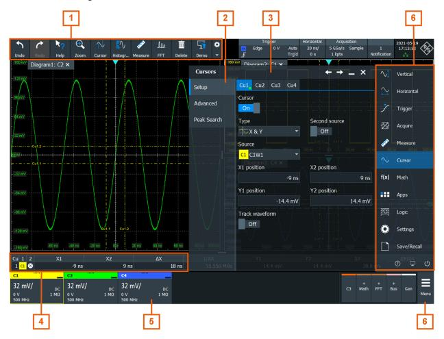
Figure 6-6: Control elements on the touchscreen
