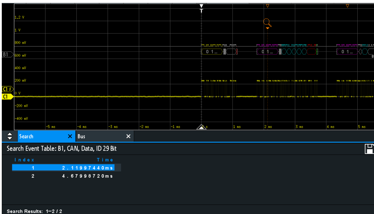
Figure 13-25: Search on a CAN bus for data frames with 29-bit ID
