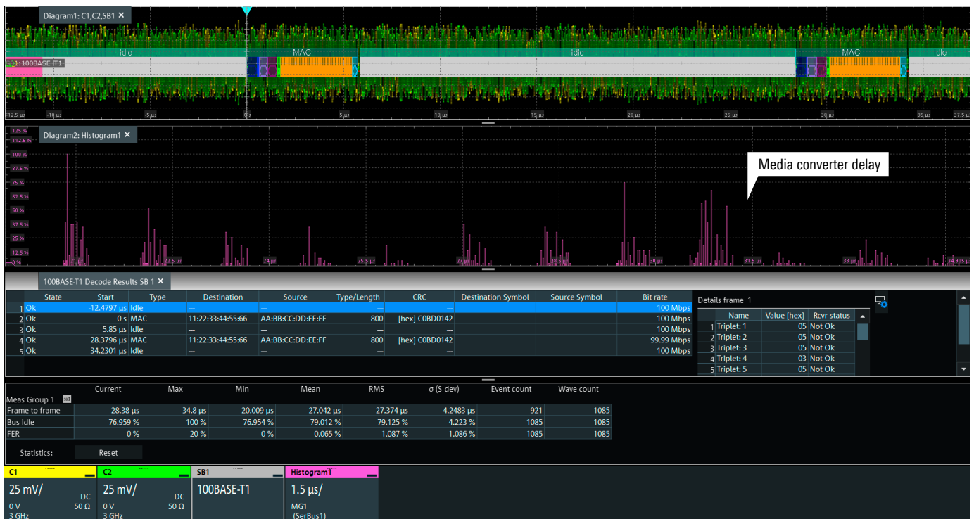
Example of bus timing measurements on a 100BASE-T1 bus
