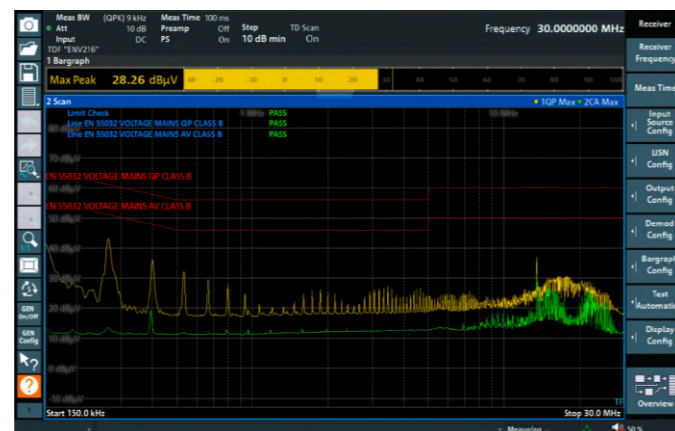
Checking a laptop power supply in CISPR band B. The measurement takes about 3 s for one mains line with a measurement time of 1 s. All signal components are captured seamlessly in the same timeframe.
