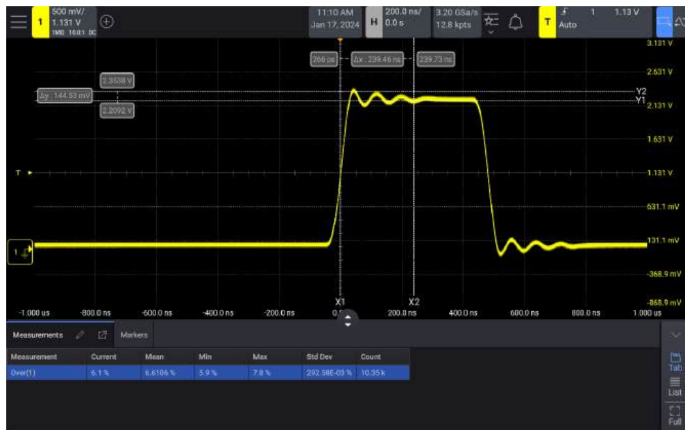
Figure 41 Automatic Overshoot measurement
