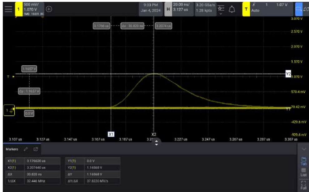
Figure 35 Markers used to measure pulse widths other than middle threshold points
