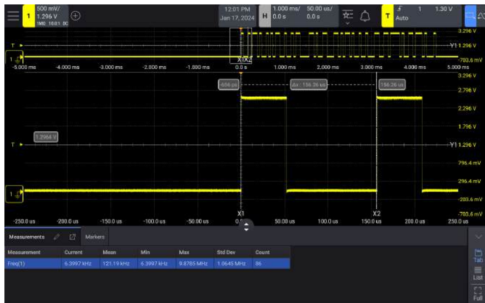
Figure 42 Isolating an event for Frequency measurement
