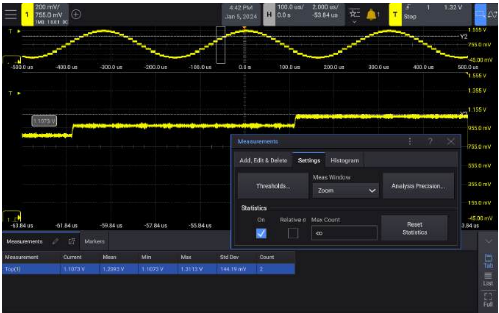
Figure 40 Isolating area for Top measurement
