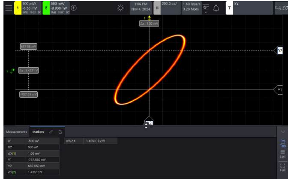
Figure 6 Phase difference measurements, automatic and using markers
