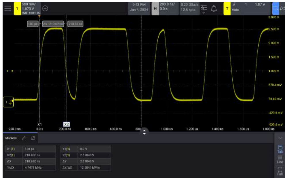
Figure 38 Measuring pulse width with markers
