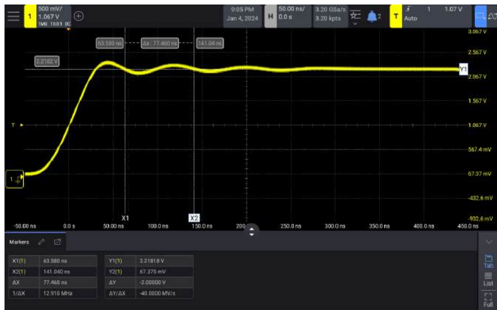
Figure 36 Markers measure frequency of pulse ringing
