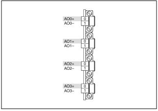
Figure 2. NI 9269E Terminal Assignments
