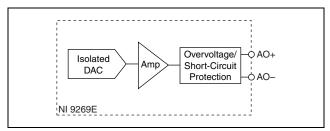
Figure 4. Output Circuitry for One Channel of the NI 9269E
