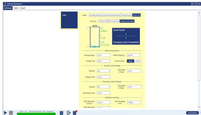
Cycle Test Batteries using constant current, constant voltage, or hybrid CC + CV charge.
