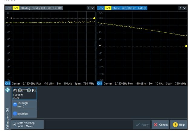
The analyzer performs a calibration sweep for the measured quantity  $S_{21}$ . The magnitude and phase of the result is displayed in two diagrams, together with the expected typical result for a Through standard. The similarity of real and expected traces indicates that the Through standard has been properly connected. After the R&S ZNL has completed the calibration sweep and calculated the correction data, the "Apply" button is enabled.
