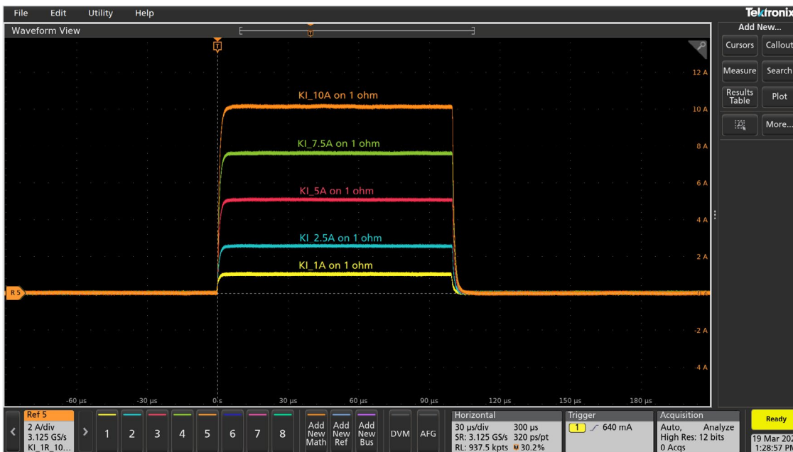
Figure 7: 2601B-PULSE 100 μs amplitude sweep at 1, 2.5, 5, 7.5, and 10 A.
