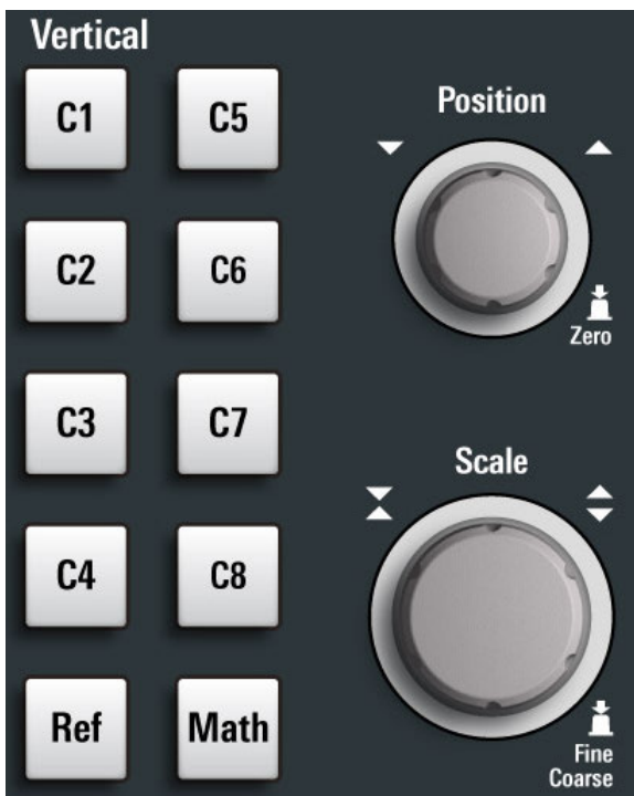
Figure 4-5: Vertical controls of R&S MXO 5 with 8 input channels
