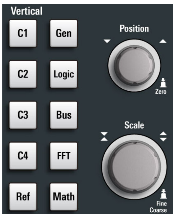
Figure 4-4: Vertical controls of R&S MXO 5 with 4 input channels
