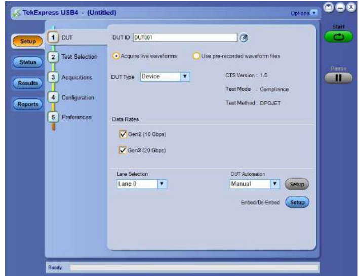
TekExpress® USB4 Automated Test Software (Option USB4) - The TekExpress® USB4 Compliance and Debug solutions provide an easy way to validate and characterize the emerging USB4 Router-Host, USB4 Router-Device, and USB4 Hubs as per the USB4 Electrical Compliance Test Specification (CTS). Tektronix MSO/DPO70000DX and DPO70000SX Series Oscilloscope (bandwidth ≥ 23 GHz) supports the Tektronix USB4 Compliance and Debug solutions.
