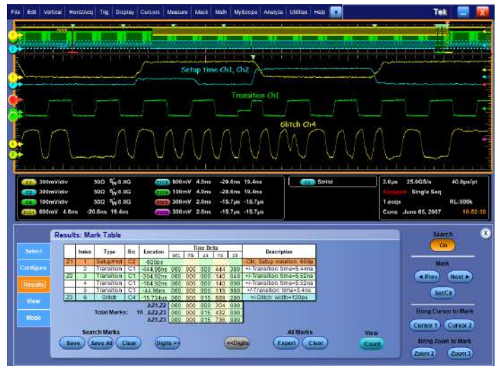
Advanced Search and Mark - Highlights important events and provides convenient previous and next buttons and mouse clicks to navigate between events of interest effortlessly
