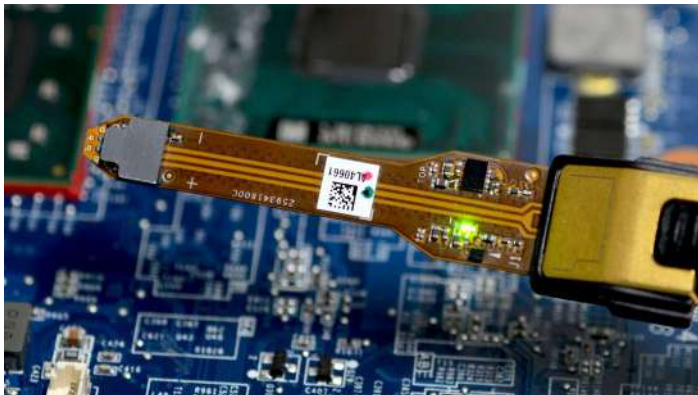
P77STFLXA solder down, flex circuit accessory with an active buffer amplifier on its tip provides up to 20 GHz bandwidth.
