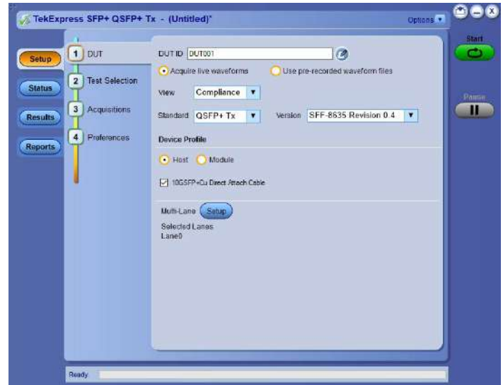
TekExpress SFP+ QSFP+ Tx (Options SFP-TX, SFP-WDP) - TekExpress SFP+ QSFP+ Tx is developed on a Real Time Oscilloscope platform, which is the platform of choice for engineers designing their products around SFF-8431 & SFF-8634 technology. Option SFP-TX and SFP-WDP enable both an Automation Solution (for Compliance) and DPOJET Option (for Debug). Users can save up to 80% on testing time compared to manual testing. TWDPc - Transmitter Waveform Distortion Penalty for Copper Measurements are available with Option SFP-WDP. SFF-8431 SFP+ TWDPc based Matlab code is integrated into the SFP-WDP option to make sure Engineers can use this measurement in the automated setup.
