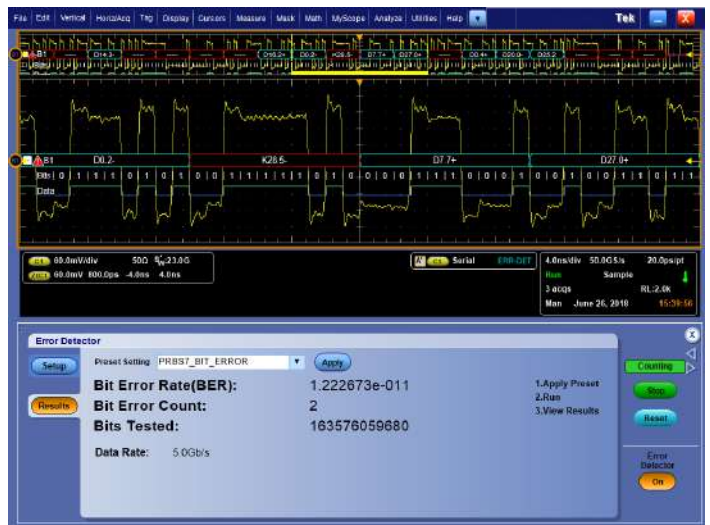
Bit Error Detector (option BITERR) - Provides statistics on bits counted and number of errors detected, as well as displaying waveform data upon detection of a bit error. As shown here, the Bit Error Detector can be combined with optional serial data decoders to facilitate debug and diagnosis of errors.
