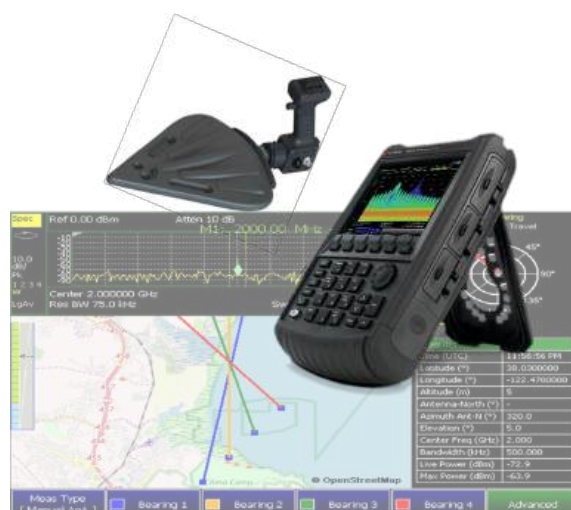
TDOA Windows PC software KSMS calculates the intersection of the hyperbolas and determines the geo-location of the RF signal source
