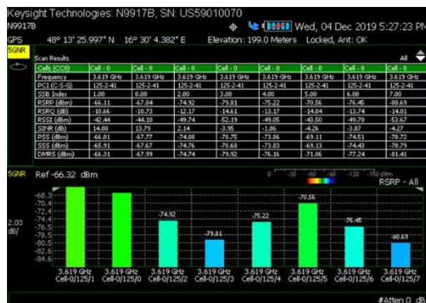
5G NR OTA measures control channels and displays cell ID
