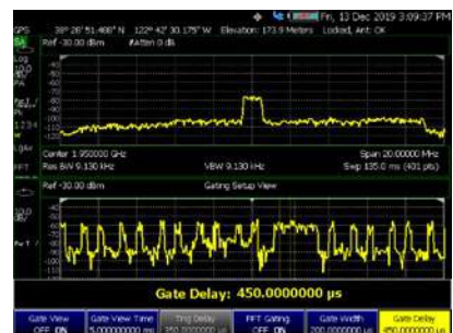
LTE FDD control channel captured with periodic frame trigger synced to GPS
