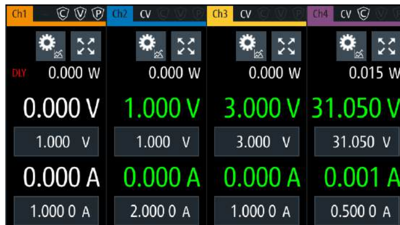
Figure 5-7: Delay text at channel display area
