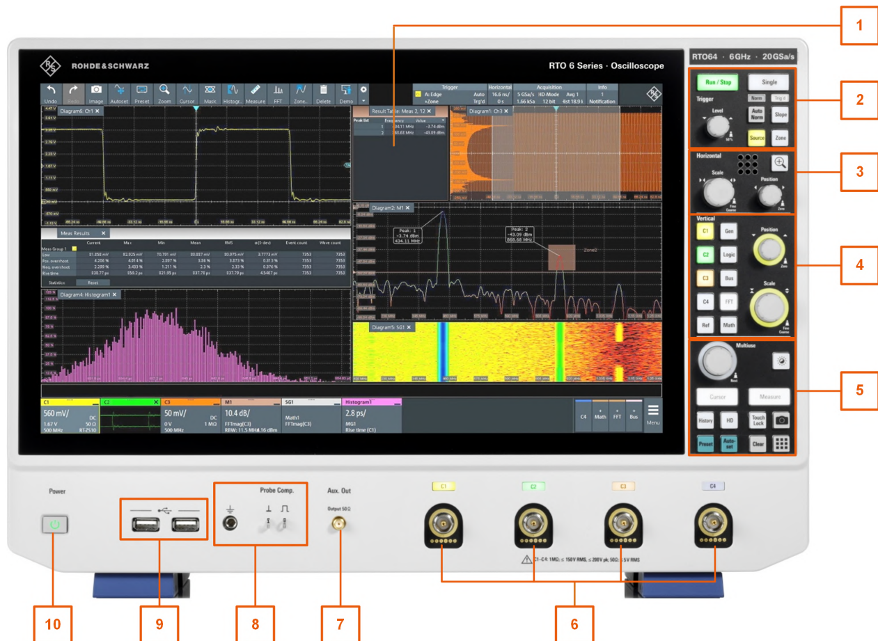
Figure 5-1: Front panel of R&S RTO6
