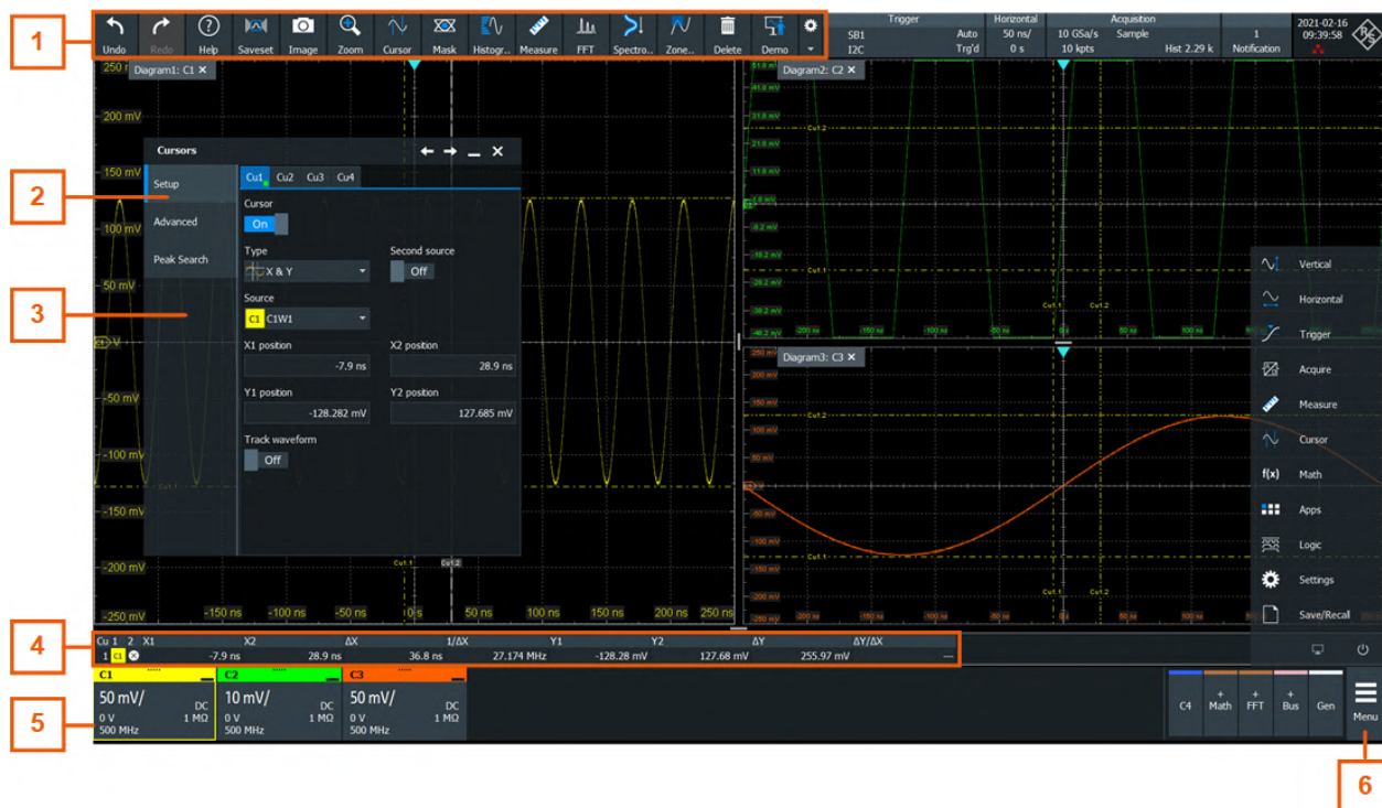
Figure 6-6: Control elements on the touchscreen
