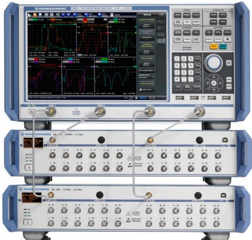
Figure 4-27: R&S ZNB connected to two R&S ZN-Z84, each equipped as 2x24 matrix
