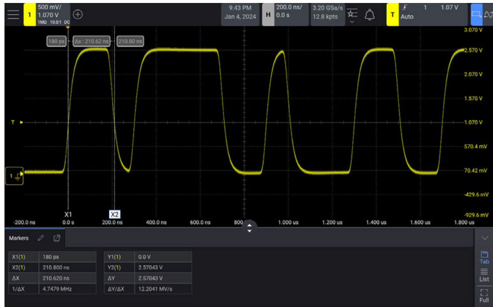
Figure 36 Measuring pulse width with markers
