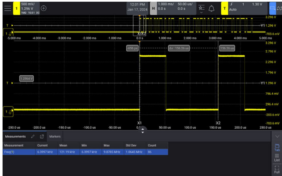
Figure 40 Isolating an event for Frequency measurement
