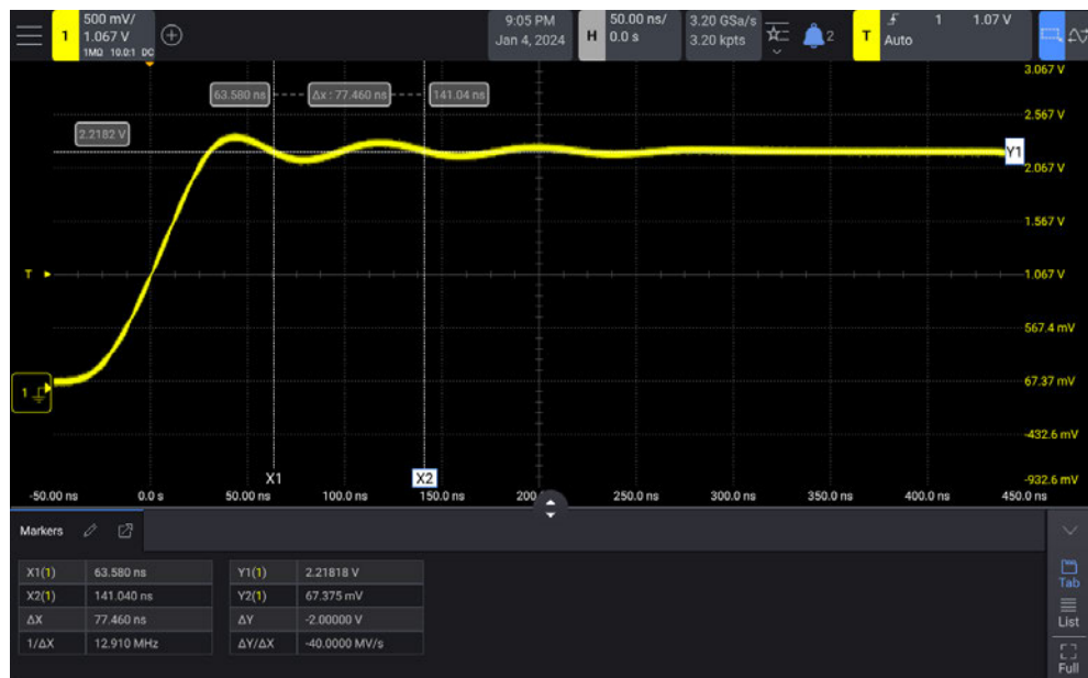
Figure 34 Markers measure frequency of pulse ringing
