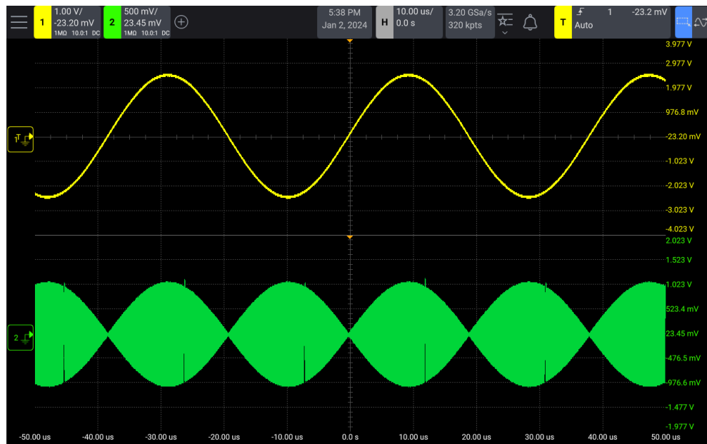
Figure 24 Amplitude Modulation Shown at 100% Intensity
