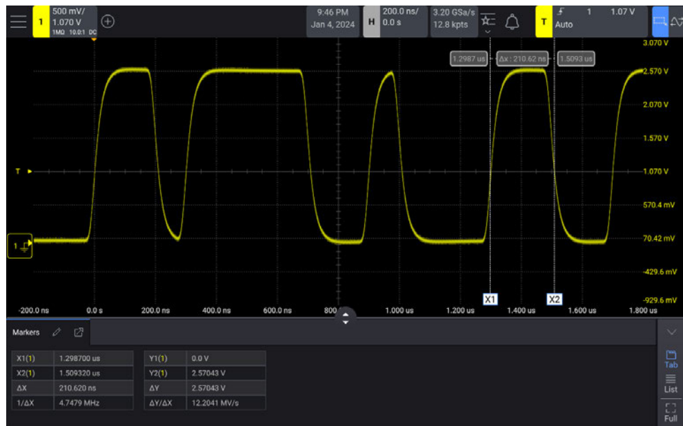
Figure 37 Moving the markers together to check pulse width variations
