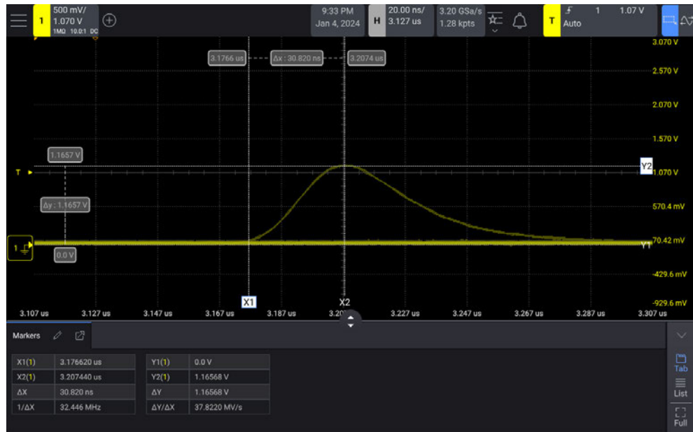
Figure 33 Markers used to measure pulse widths other than middle threshold points
