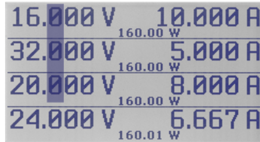
Figure 5-2: Changing the 100 mV position for three channels with the tracking function
