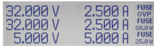
Figure 5-6: Overvoltage protection (example R&S HMP2030)
