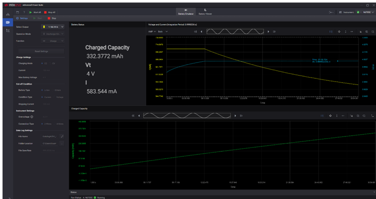
Figure 8. PW9253A Performing a battery charging on an iron phosphate battery
